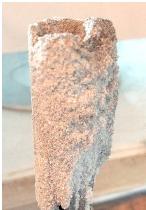
Figure 12. Agglomerated sand particles in the reaction zone of the IHFBR after combustion of coal with a sodium bearing sorbent.
